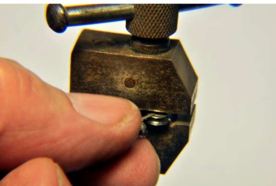
(13) Complete insertion of crank pin by squeezing assembly in jaws of vice; do NOT press in too far and cause rods to bind.
