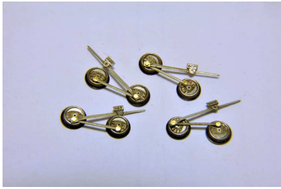
(15) Rods and driver subassemblies; note slight offset bent into main rod to assure clearing crank pin in front axle.
