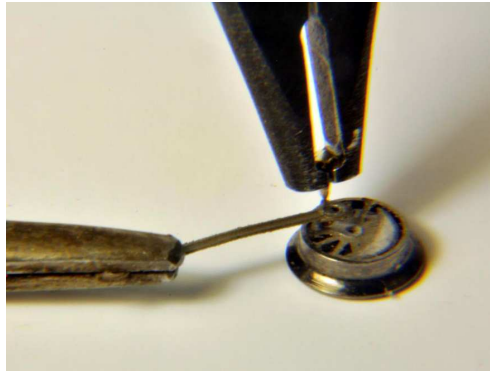
(12) Press crank pin into hole in driver through hole in etched rod.
