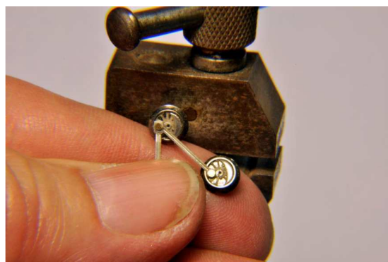
(14) Crank pins pressed into drivers through side rod and main rod; there should be a little slop in the assembly.
