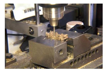
Drill holes at dimple locations (4) with #65 or 1mm drill. Hole should be all the way through at each location.
