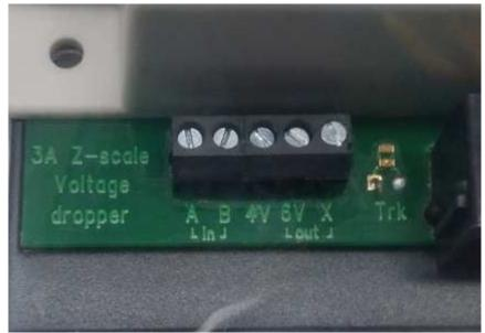
Closeup View Of The Digitrax UP-6Z Voltage Reducer Terminal Block
