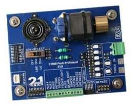
ESU 51900 LokTester DCC Decoder Test Station
